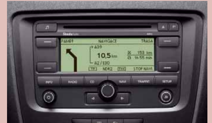
The Cruise navigation system supports map data on the TravelPilot E platform and offers the Koridor function which under certain circumstances enables uninterrupted navigation to the specified destination even when the navigation CD is ejected. It is also MP3-compatible. (AAN 600 001)
