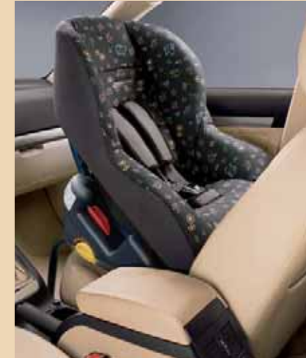
ISOFIX G 0/1 (DDF 000 009 rear-facing fittings, DDF 000 008 forward-facing fittings) Child seat frame fittings (DDF 000 003 rear-facing fittings, DDF 000 002 forward-facing fittings)
