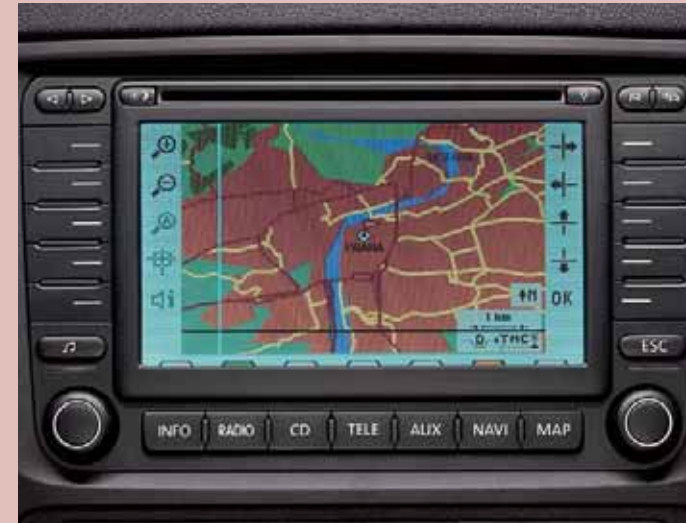
The Nexus navigation system based on the DX platform with the dynamic module (TMC) enables you to receive traffic reporting and adapt your route to up-to-date information. Of course you can also use it to play CDs and connect a CD changer. (AAN 600 002)
