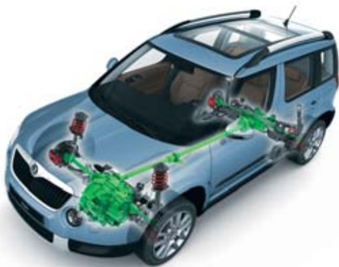
ŠKODA Yeti with four-wheel drive, latest generation Haldex clutch and 103TDI diesel engine or 112TSI petrol engine.
