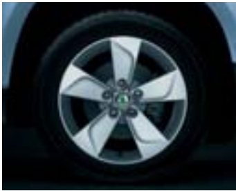
Nevis 7.0J x 16" alloy wheels for 215/60 R16 tyres are standard on the 4x4 models.
